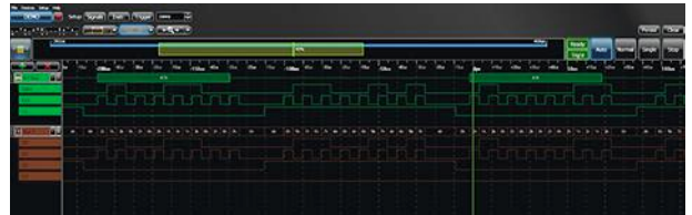
3. This logic-analyzer display shows a four-wire digital bus (D0-D3) and the three component signals of an SPI serial interface data (DATA), clock (CLK), and chip select (CS). The digital bus state (BUS1) is displayed along with the SPI bus decode (SPI Bus). (Source: ClariTek, using Teledyne LeCroy LogicStudio software operating in demo mode)
